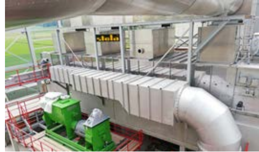
Project: Schwenk Zement KG Country: Germany Type: BTL 1/3000-14 Product: RDF Water evaporation capacity: 8.9 t/h from 15% - 5% MC
