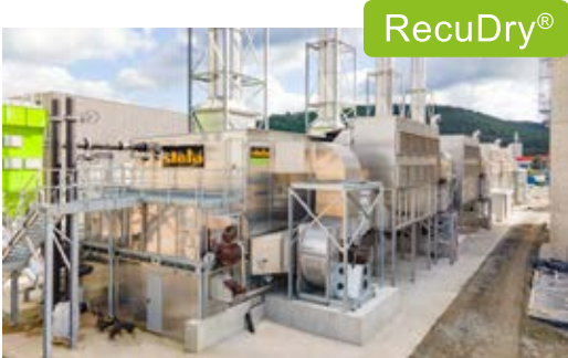
Project: Ziegler Country: Germany Type: BTU RecuDry 1/6200-60 Product: sawdust Water evaporation capacity: 36.4 t/h from 40% - 10% MC
