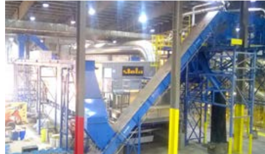
Project: Edmonton Waste Management Country: Canada Type: BTU 1/6200-18-3-2 Product: RDF Water evaporation capacity: 4.1 t/h from 40% - 10% MC
