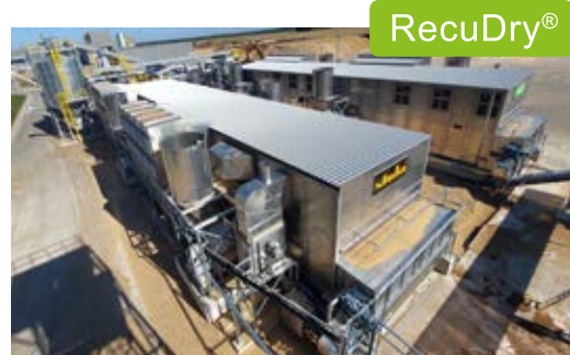
Project: VGM Country : Lithuania Type: 2 X BTU RecuDry 1/6200-34.5 Product: Wood Chips Water Evaporation Capacity: 14 t/h from 47% - 2% MC
